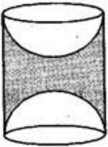
**Ans.** TSA of the article =  $2\pi rH + 2(2\pi r^2)$  = curved surface area of cylinder + curved surface area of 2 hemispheres
